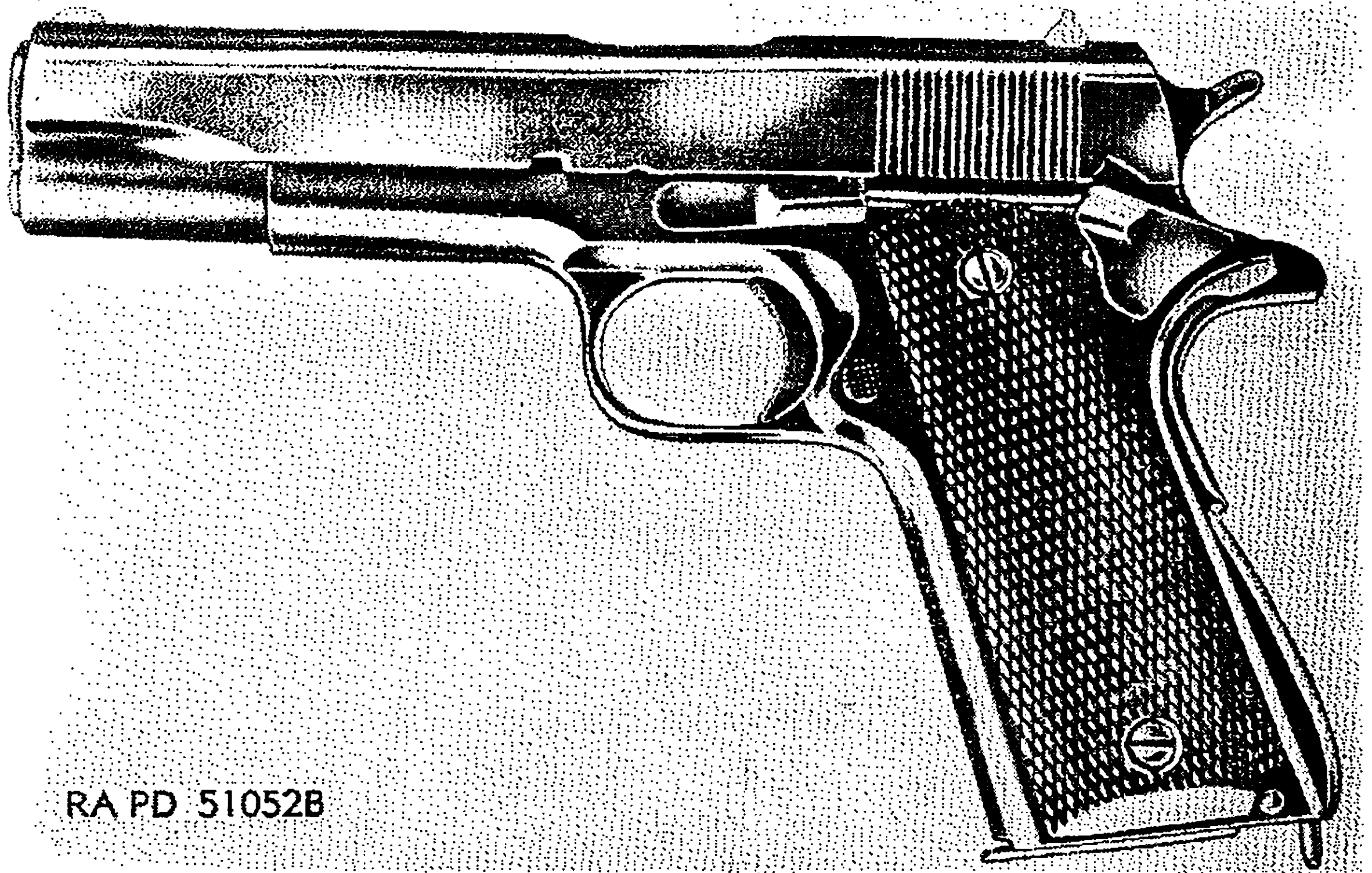
Figure 4. Cal. .45 automatic pistol M1911A1—left side view.
