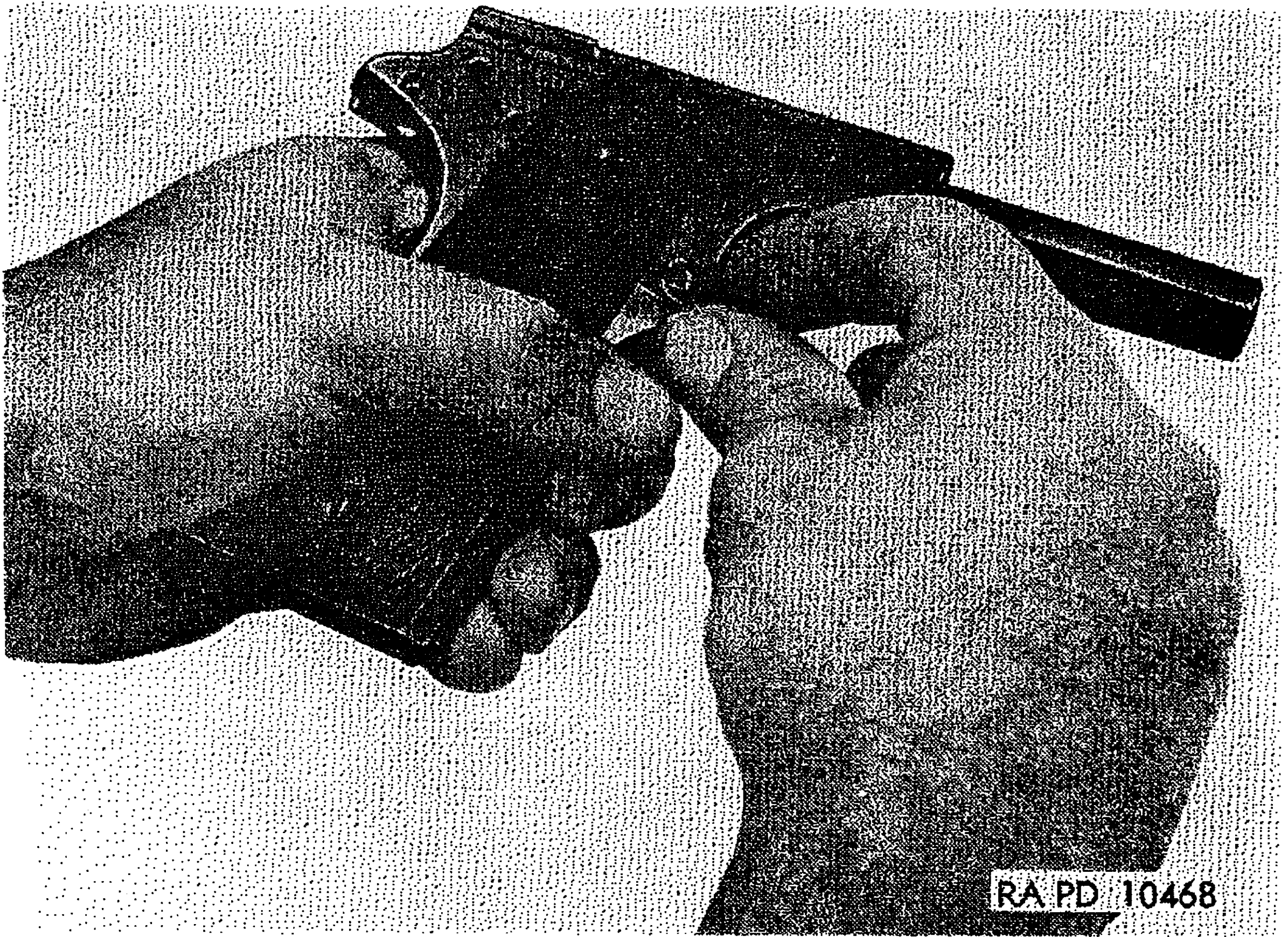
Figure 36. Removing old design magazine catch from receiver.
