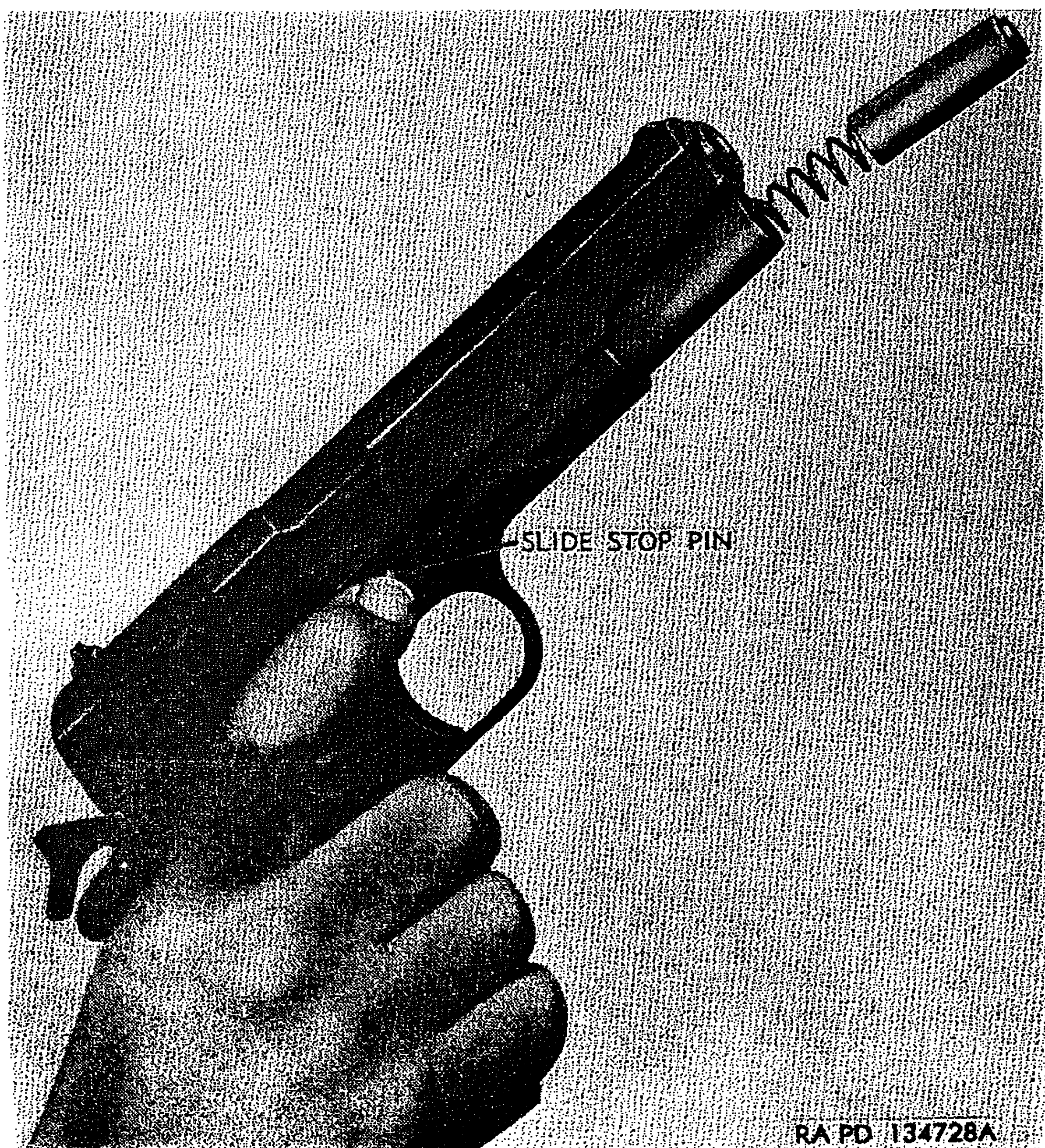
Figure 23. Disengaging slide stop pin.
