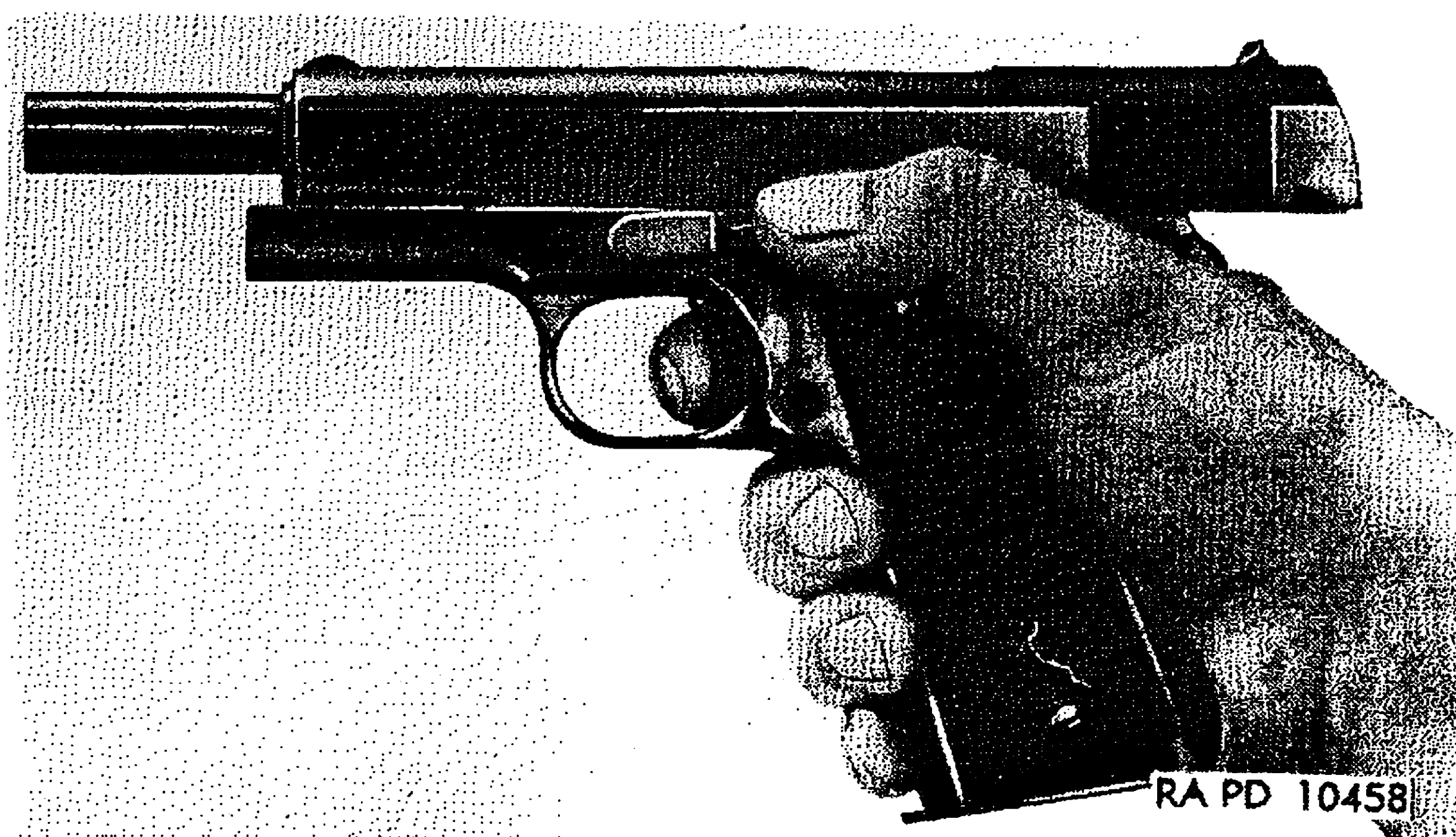
Figure 18. Disconnecter test pistol M1911A1, slide fully back, slide stop engaged, thumb releasing slide, hammer back.
