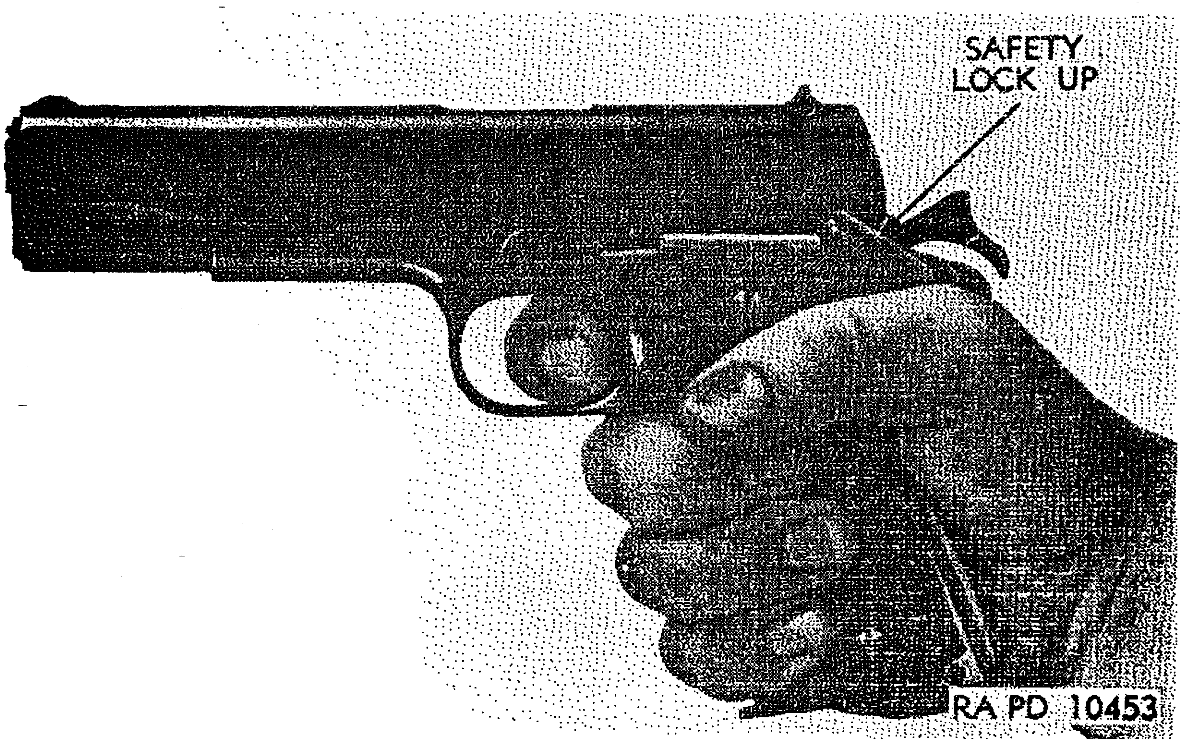
Figure 13. Pistol M1911A1, hammer back, safety lock upward in safe position, hand grasping stock so grip safety is depressed, finger squeezing trigger.
